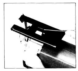
Loosen the bolt on the back of the base with the hex wrench, and slide the base backwards. Tilt the base to the desired angle. The edge of the housing indicates the bevel angle. Then check for contact between the back edge of the blade and the roller.
